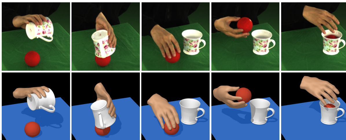
Figure 1: Modeling high-fidelity dexterous manipulation data from videos: (top) observed image data; (bottom) reconstructed motion.
