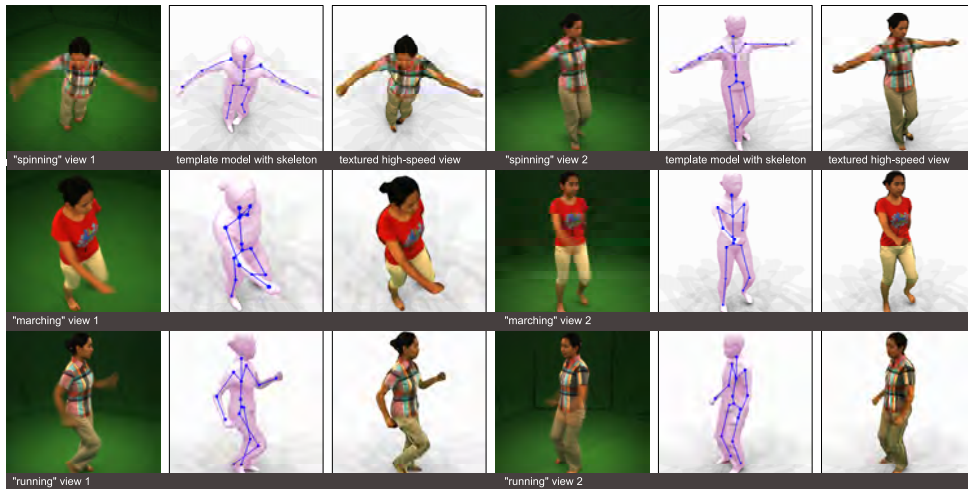
Figure 9: Results for three different reconstructed performances (see also accompanying video). Each row shows two results from two different viewpoints. From left to right: captured blurred image, one of the reconstructed high-frame rate models with the skeleton, model with deblurred texture.
