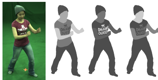
Figure 5: Average BRDF per material segment. (a) Input image, (b) diffuse albedo, (c) specular albedo (both for red channel), (d) specular exponent. All values are scaled to [0.3, 0.8] , and shown in gray scale. Note the plausibly captured high specularity of the print on the t-shirt.
