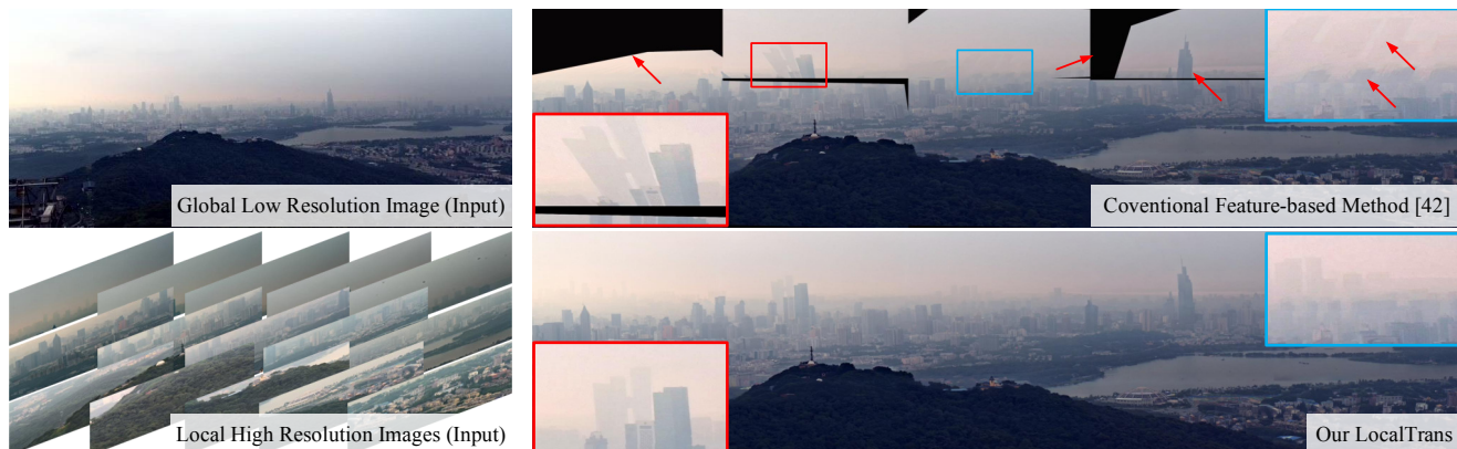
Figure 1. We present a multiscale local transformer network, dubbed LocalTrans , for homography estimation. The proposed LocalTrans network achieves accurate homography estimation on challenging real-captured cross-resolution cases under resolution gap up to 10\times . By warping each of the local high-resolution image on a global low-resolution image using the estimated homography matrix, we achieve artifact-free stitching on this challenging case, substantially outperforms feature-based homography estimation in [42].
