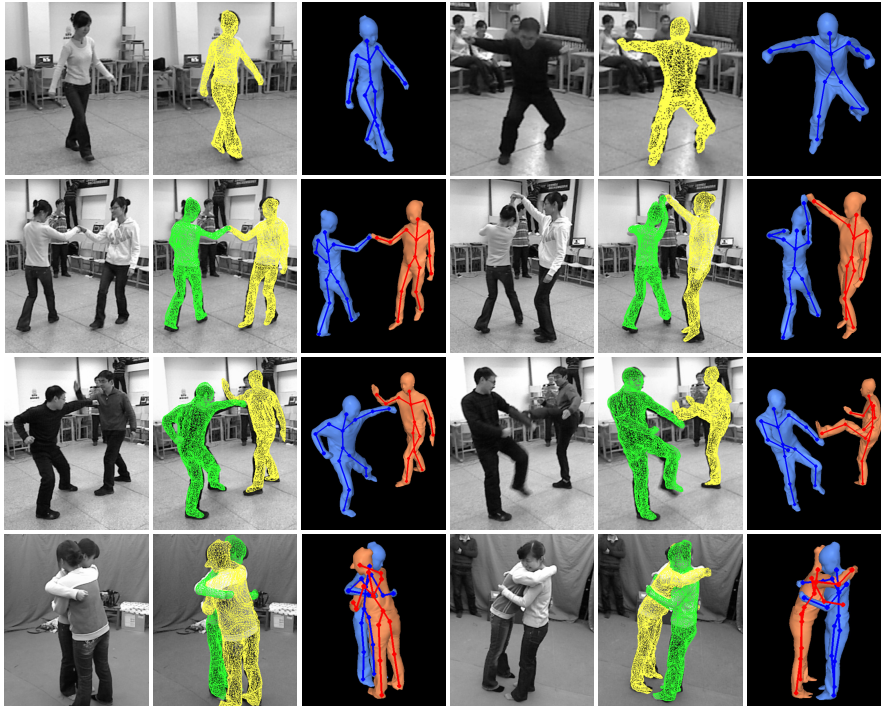
Fig. 5. Performance capture results on a variety of sequences: input image, deformed mesh overlay, and 3D model with estimated skeleton respectively.
